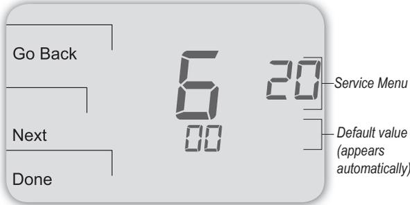
3. In Service Menu 620, press ▲ / ▼ to select option "01" to enable fan output (see Fig. 13).
